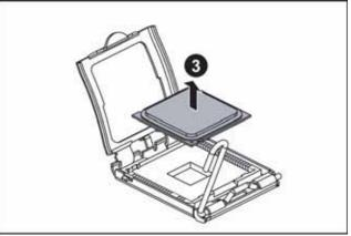
8 Insert the new processor into the socket, making sure that the gold triangle on the corner is situated as shown in the following illustration.
